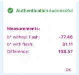
The app developed by Ara-Authentic measures the color values b\* at a specific location, once without and once with a flash. Only if the difference between the two color values is greater than 80 is the sample considered an original.
